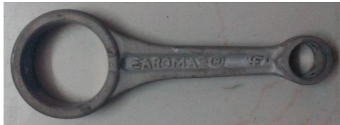
Fig. 5.2 Connecting rod with 3g Ni-TiO 2 Composite Coating
