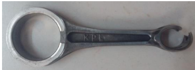
Fig. 5.5 Uncoated connecting rod after tensile test
