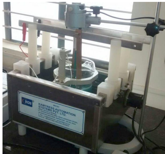
Fig. 2.2 Electrocodeposition equipment during coating process
