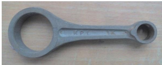
Fig. 5.16 9g coated connecting rod after corrosion test
