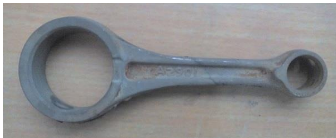
Fig. 5.15 6g coated connecting rod after corrosion test
