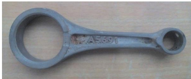
Fig. 5.14 3g coated connecting rod after corrosion test
