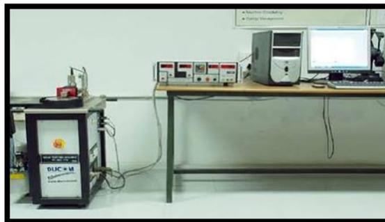
Figure 1: Pin on Disc Machine
