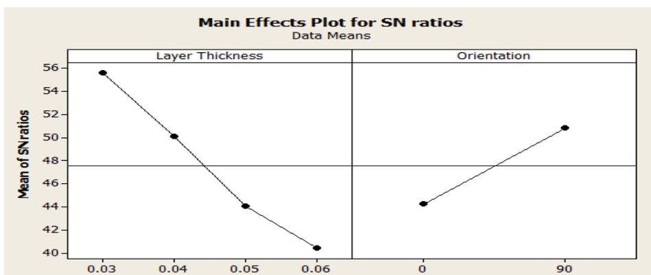
Fig. 4- Effect of control factor on width
