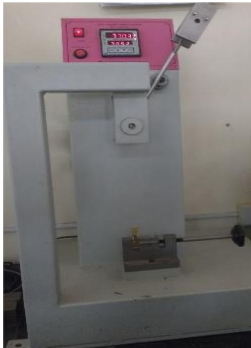
Figure 4.12 Izod impact test
