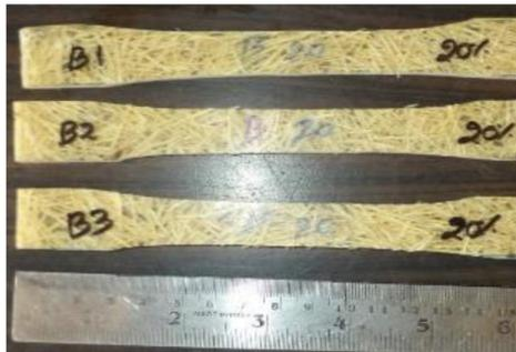
Figure 4.6 Tensile test specimen
