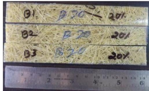
Figure 4.7 Flexural test specimen
