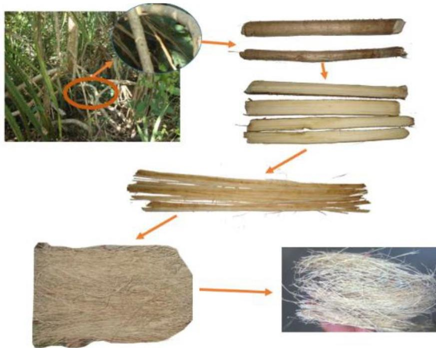
Figure 2.1 Fibre extraction process in brief
