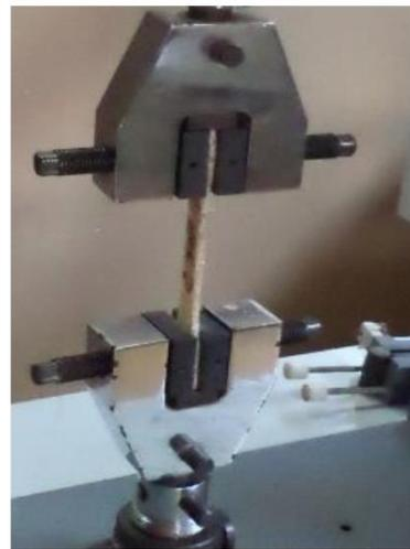
Figure 4.10 Tensile specimen
