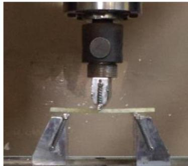
Figure 4.11 Specimen during flexural test
