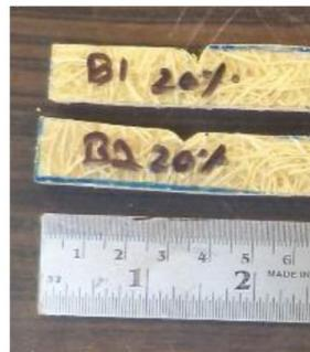
Figure 4.8 Izod impact test specimen
