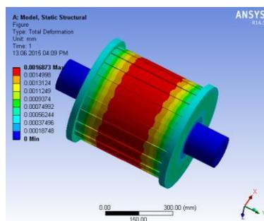
Figure 2.6 Total Deformation
