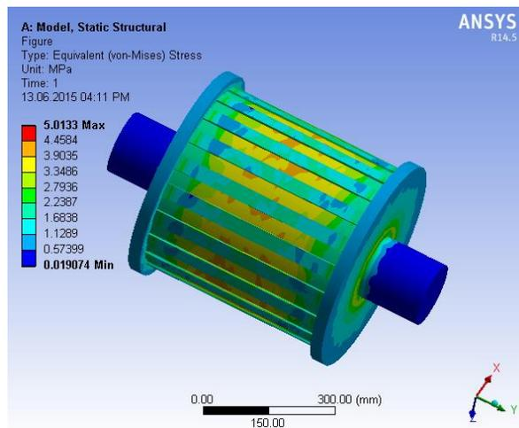
Figure2.5 Equivalent Stress
