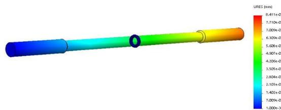
*Fig.6 Deflection Plot for Butt Welded Specimen*
