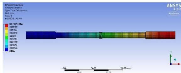
*Fig. 8 Deflection Plot for Butt Welded Specimen in ANSYS*
