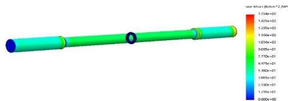
*Fig.5 Stress Distribution in Butt Welded Specimen in solid works*
