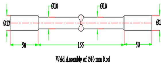
*Fig. 2 Schematic representation of welded joint*
