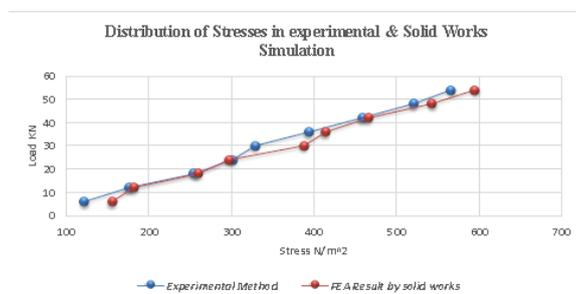
*Fig. 9 Stress plot for experimental and solid works Simulation*
