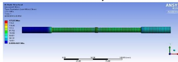
*Fig.7 Stress Distribution in Butt Welded Specimen in ANSYS*
