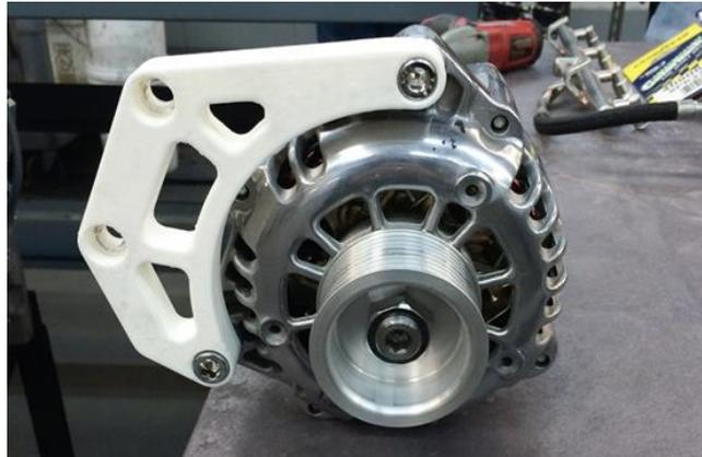
**A functional alternator bracket printed using SLS nylon**
