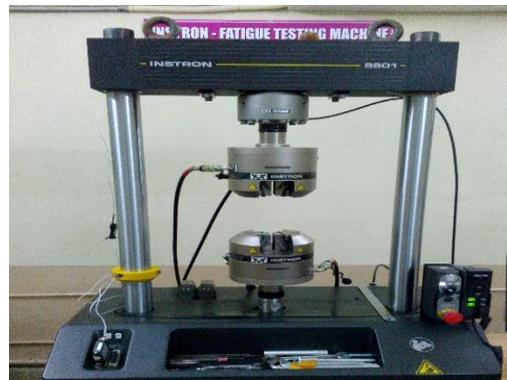
Fig.2.2 Universal Hydraulic Fatigue Testing machine
