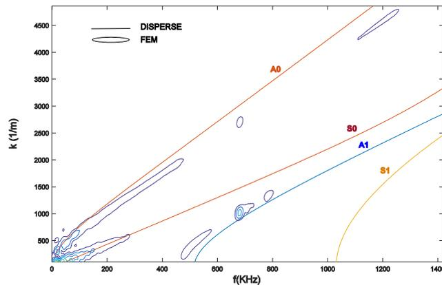
**Figure 7:** Comparison between FEM and DISPERSE dispersion curves.
