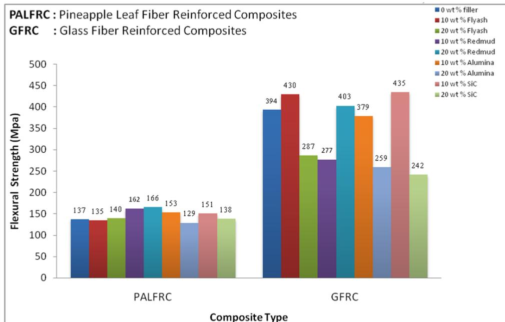
Figure 4.4 Flexural strength of composites with different particulate fillers
