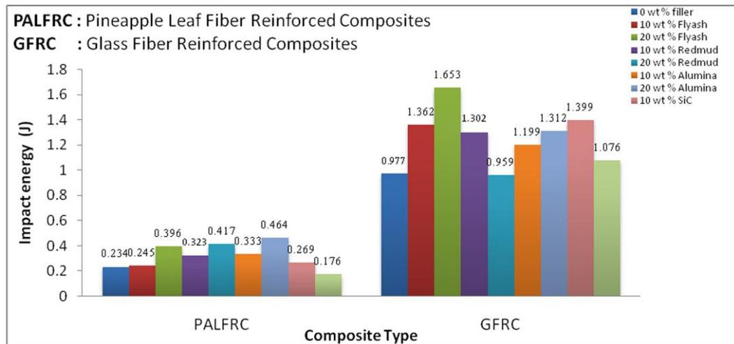
Figure 4.6 Impact strength of composites with different particulate fillers
