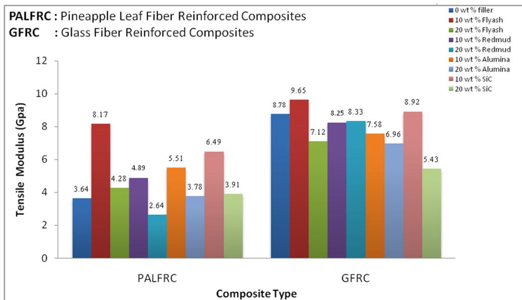
Figure 4.3 Tensile modulus of composites with different particulate fillers
