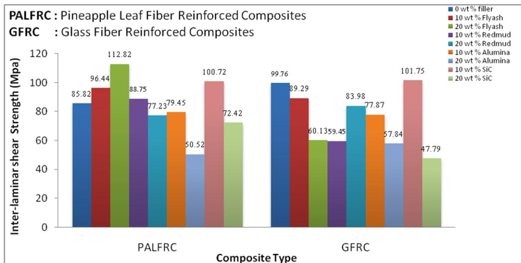
**Figure 4.5** Inter-laminar shear strength of composites with different fillers
