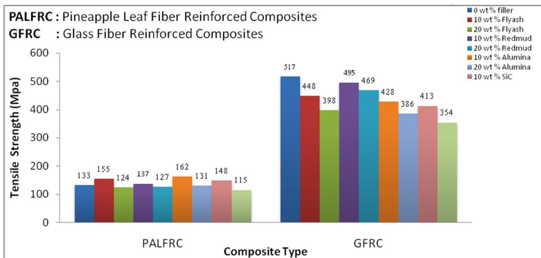
Figure 4.2 Tensile Strength of composites with different particulate fillers
