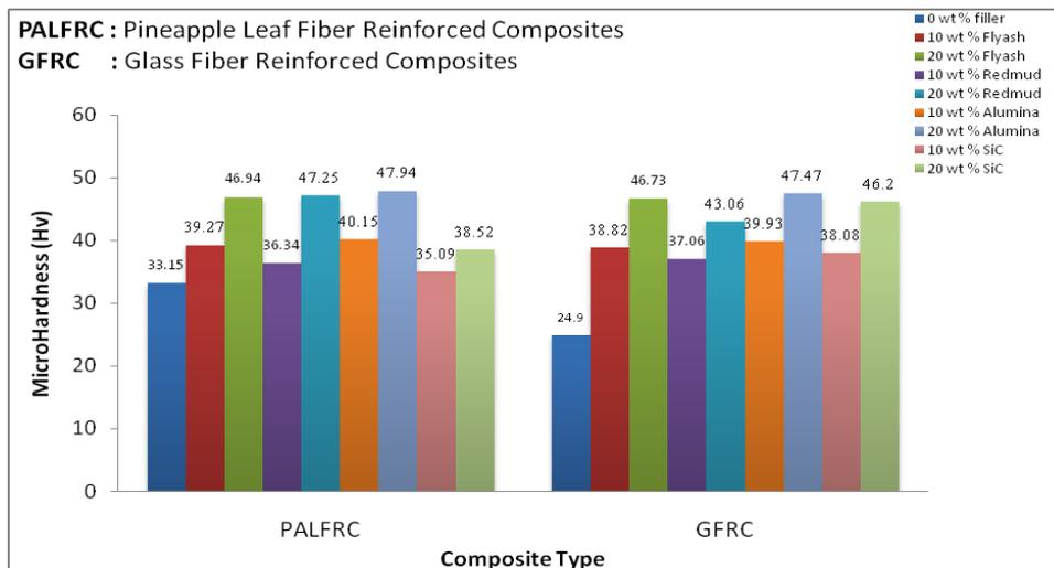
Figure 4.1 Micro-hardness of composites with different particulate fillers
